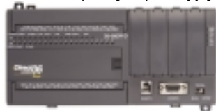
DO-06AA AC in/AC out/AC supply
