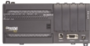
DO-06DR-D DC in/Relay out/DC supply
