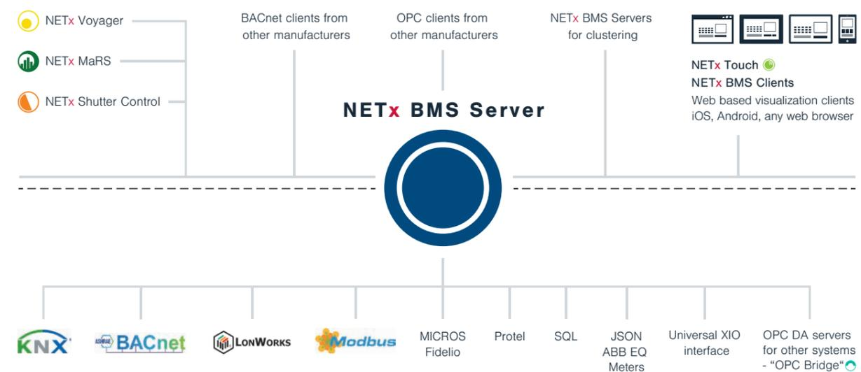
The NETx BMS Server is the core component for solutions within the building management domain. As a server application it is responsible for collecting and processing datapoint values from any building automation system. The datapoints themselves can originate from a variety of systems and technologies. The NETx BMS Server offers the possibility to integrate datapoints from KNX, Modbus, LonWorks or BACnet. In addition, interfacing to other systems is possible too.
