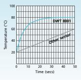
**Sensor crown** – ensures good thermal contact with the end of the pocket using a pre-applied heat paste which conducts the heat directly to the thermistor. Fast response DWT 0002 –
