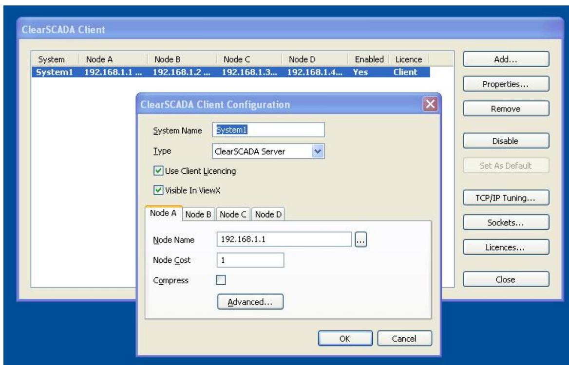
The previous section described how a ViewX workstation is connected to the ClearSCADA server or a set of servers if in a redundant arrangement. This concept can be further extended by connecting the ViewX workstation to multiple systems or databases, a term we call 'clustering'. All that is involved to do this is add another entry in the ClearSCADA Client Configuration program for each system that you wish to connect to.
