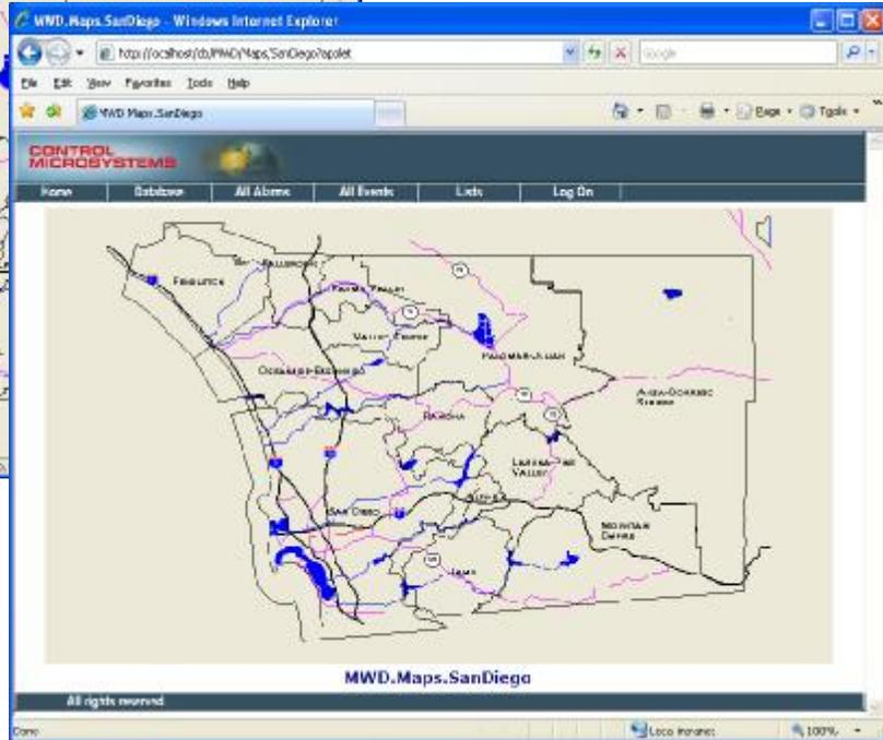
The ClearSCADA Web server defaults to the IP address of the ClearSCADA server and supports XML and/or html with optional secure sockets (SSL) for added security if necessary.
