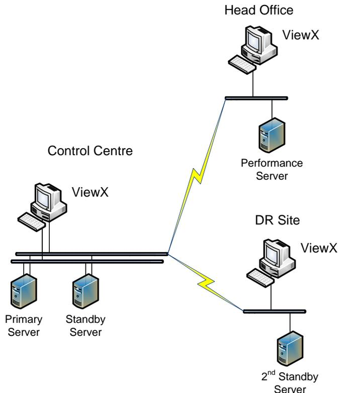
The configuration of the server setup in a redundant arrangement is a simple matter to fill in the form as shown to the right. All that is necessary is to specify the Name/IP address for the servers and restart the application. Redundancy is an integral function of ClearSCADA without the need of 3<sup>rd</sup> party software.
